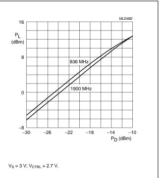
Fig.4 Load power as a function of drive power; typical values.
