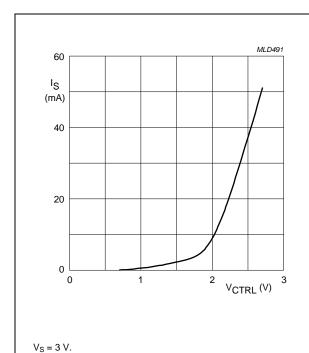
Fig.3 Total supply current as a function of control voltage; typical values.
