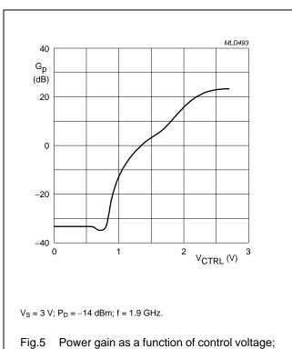
Fig.5 Power gain as a function of control voltage; typical values.
