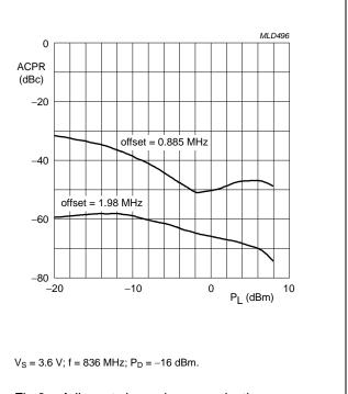
Fig.8 Adjacent channel power rejection as a function of load power; typical values.
