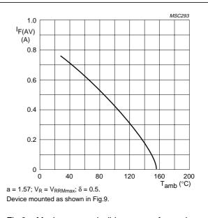
Fig.3 Maximum permissible average forward current as a function of ambient temperature (including losses due to reverse leakage).
