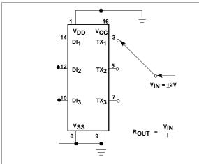
Figure 1. Power-Off Source Resistance (Drivers)
