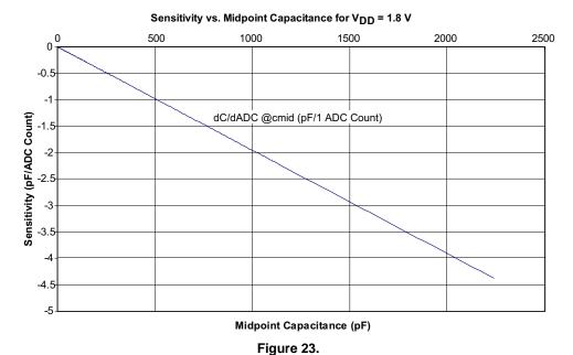
Smaller amounts of change indicate increased sensitivity for the capacitance sensor. Some sample values are shown in Table 11.
