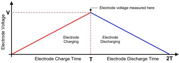
Figure 21. MPR03X Electrode Measurement Charging Pad Capacitance
