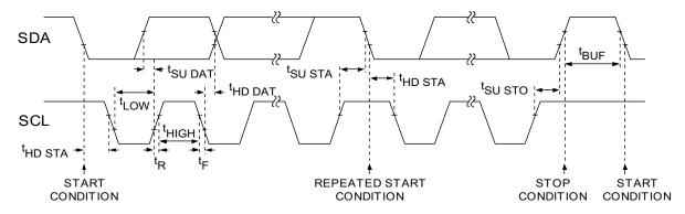
Figure 5. Wire Serial Interface Timing Details
