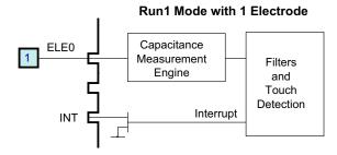
Figure 14. Electrode/Pad Connections in Run Mode
