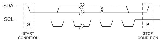
Figure 7. Stop and Start Conditions
