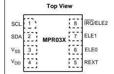
Figure 1. Pin Connections
