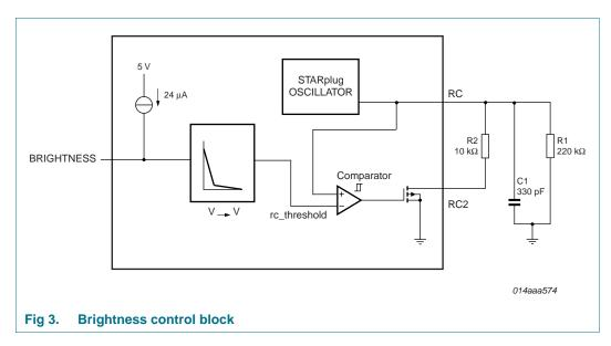
A typical RC waveform is given in  $\underline{\text{Figure 4}}$ . The RC switch-over threshold is controlled by the BRIGHTNESS pin.
