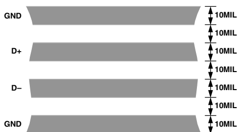
Figure 8. Arrangement of Signal Tracks
