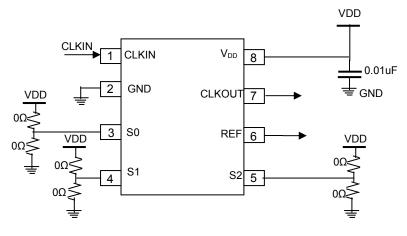
Use either pull-up or pull-down  $0\Omega$  Resistor with [S2:S0] for selection of CLKOUT frequencies.
