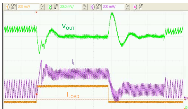
Figure 22. Load Transient 150mA to 400mA, V_{IN}=3.6V , t_{RISE}=t_{FALL}=100ns , 5μs/div.
