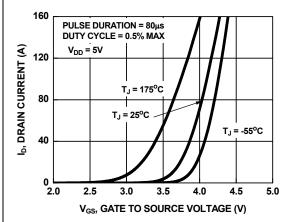
Figure 7. Transfer Characteristics
