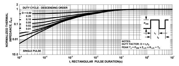
Figure 3. Normalized Maximum Transient Thermal Impedance
