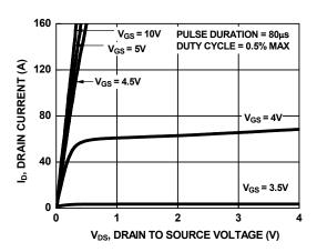
Figure 8. Saturation Characteristics
