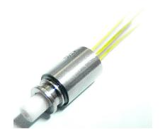
The FP-1310-4I-LCx is an MOCVD grown InAlGaAs ridge laser diode with emission wave-length of 1310 nm and standard continuous light output of 5mW per facet. These lasers provide stable, single transverse mode oscillation.
