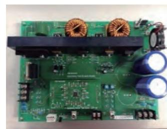
IGBT loss is reduced by fast switching performance.
