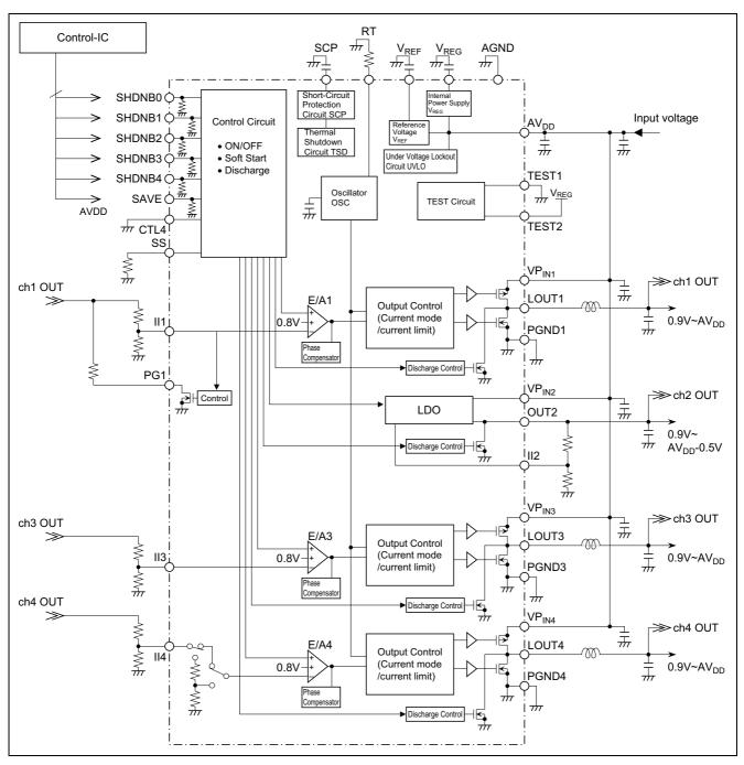
ch1 to ch3: Adjustable output voltage by external resistor. ch4: Adjustable output voltage by external resistor is selected. (CTL4 = L)
