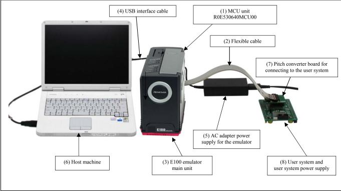
Figure 1.1 System configuration
