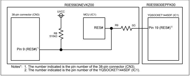
Figure 2 Reset Circuit
