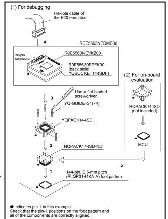
Figure 3 Connections of the User System and This Product
