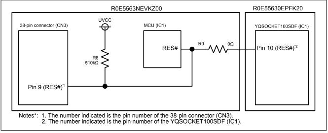
Figure 2 Reset Circuit
