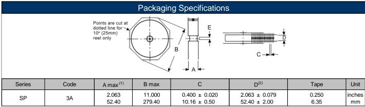
Dimension "E": This is a non-critical dimension that does not have a tolerance in the standard. Range of diameters is from 0.547 inches (13.90 mm) to 1.500 inches (38.10 mm).
