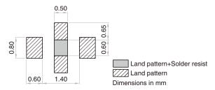
\* Make sure to connect the GND terminal of this product and the GND of the mounting circuit board by using through holes so that the distance between them is the shortest.
