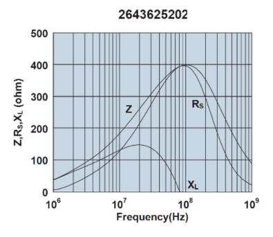
Impedance, reactance, and resistance vs. frequency.
