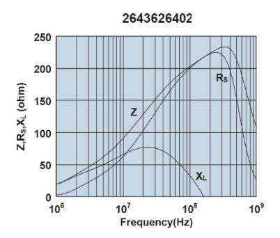
Impedance, reactance, and resistance vs. frequency.
