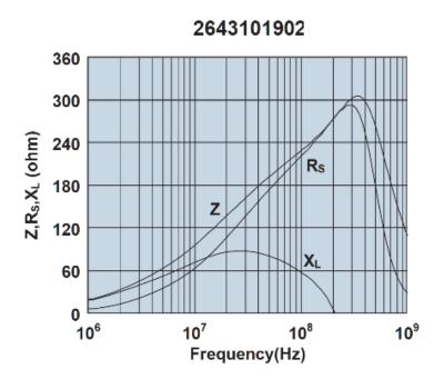
Impedance, reactance, and resistance vs. frequency.
