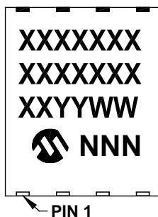
8-Lead DFN-S (6x5x0.9 mm)
