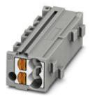
Marshalling patchboard, Nom. voltage: 500 V, Nominal current: 17.5 A, Cross section: 0.14 mm<sup>2</sup> - 2.5 mm<sup>2</sup>, AWG: 12 - 26, Connection type: Push-in connection, Number of positions: 1, Number of connections: 4, Width: 11 mm, Length: 8.6 mm, Color: gray, Color of connection elements: white, Assembly: for snapping onto a DIN rail adapter, for snapping onto a cover flange
