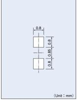
The recommended thickness of the screen mask for soldering is between 100 and  $200\,\mu$ m. The hole size of the screen mask should be same as the recommended land pattern or smaller.
