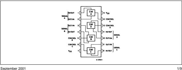
the ON resistance is relatively constant over the full input signal range. The HCF4066B consists of four independent bilateral switches. A single control signal is required per switch. Both the p and n device in a given switch are biased ON or OFF simultaneously by the control signal. As shown in schematic diagram , the well of the n-channel device on each switch is either tied to the input when the switch is ON or to  $V_{\rm SS}$  when the switch is OFF. This configuration eliminates
