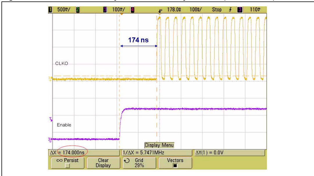
Figure 19. STCD2400 recovery time from off to on (VTCXO first in standby)
