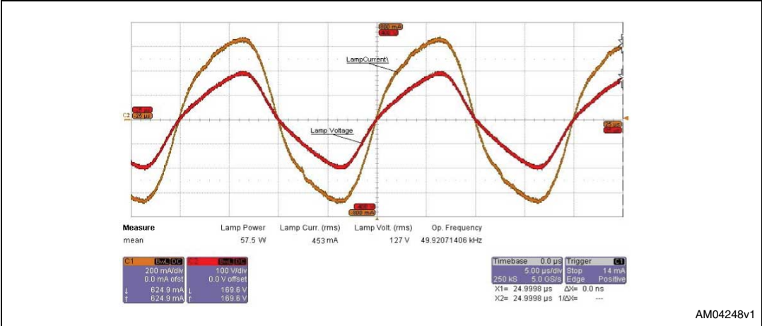
Figure 20. Steady-state lamp parameters
