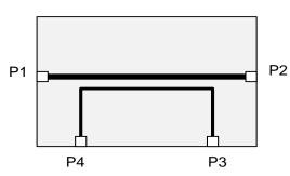
P1 : In/Output RF P2 : In/Output RF P3 : Coupled RF – P2 P4 : Coupled RF – P1
