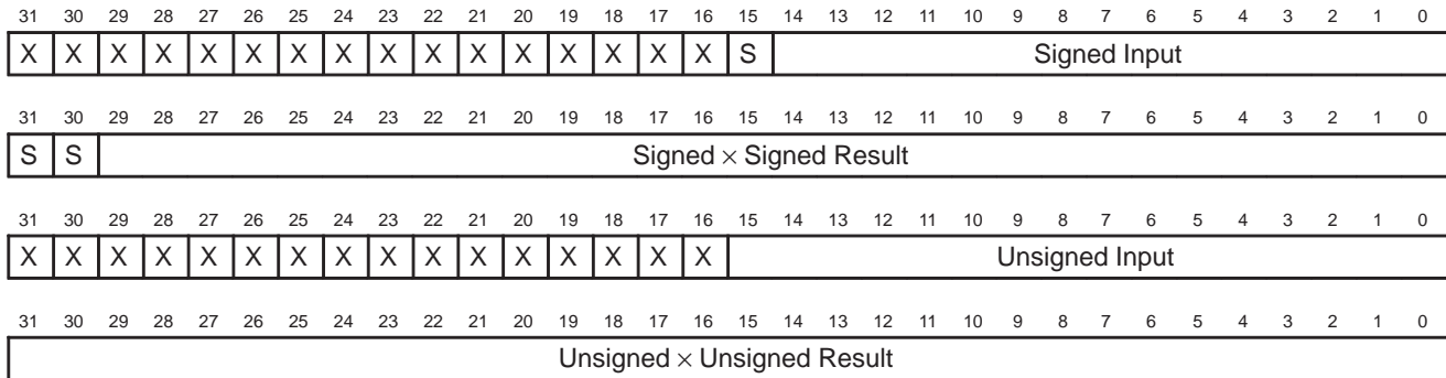
Figure 39. 16 x 16 Multiplier Data Formats
