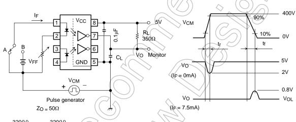
$$\text{CM}_{H} = \frac{320(\text{V})}{t_{f}(\mu s)}, \text{CM}_{L} = \frac{320(\text{V})}{t_{f}(\mu s)}$$
