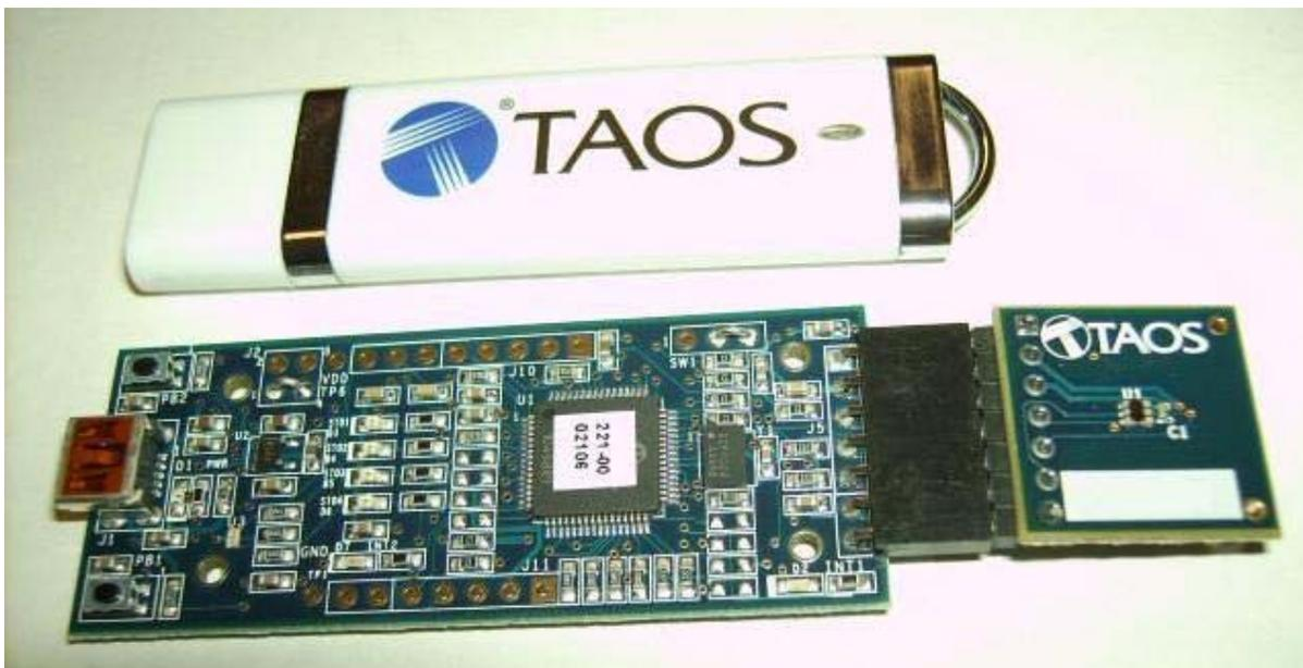
When the USB cable is first connected the green LED should light up indicating that power is being received via the USB interface, and the controller board processor is running. If the green LED does not light up check the USB cable connections unplug the USB cable and try again. If after re-try no green LED check the PC for USB error messages. See resources section at end of this document for additional assistance.
