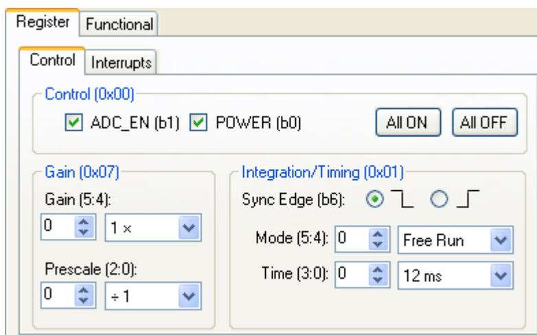
The Control sub-tab allows enabling and disabling device functionality, controlling the gain/prescale values and also controlling Integration timing and modes.
