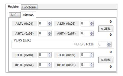
The AILT and AIHT values are 16 bit thresholds for the upper and lower trigger points. Each is set using two 8-bit registers. Another control (APERS) establishes the required persistence of the interrupt signal.
