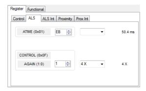
ATIME Register (0x01) controls the ALS integration time. The actual time is: (256-ATIME) \* 2.72 ms
