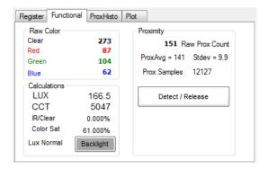
The Raw Color box displays the output register values of the Clear, Red, Green and Blue photodiodes.
