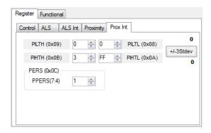
Also on this screen is a control that will automatically generate the register values to provide threshold settings 3 standard deviations higher and lower than the Proximity Data Register value. See the description of the Stdev button on the Input Side Functional tab above, for details.
