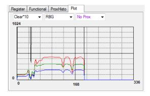
This sample graph shows all the color outputs for a typical system. The X-axis plots 337 points then rolls over back to 1 on the graph. The Y-axis is set to range 0 to 1024; this range cannot be adjusted. However Multipliers (selected from the list boxes) may be used to scale the display accordingly.
