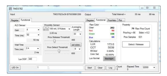
This window has inputs organized on the left, and outputs organized on the right. Values for register variables may be set using multiple techniques. The Functional tab is commonly used to quickly evaluate the device with nominal settings. The Input Register tab allows the register settings to be changed, and the Output Register tab allows registers to be viewed. Other tabs provide additional demonstration and test features for evaluation.
