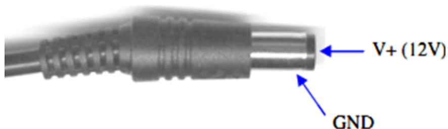
Figure 2. 2.1 mm Power Connector
