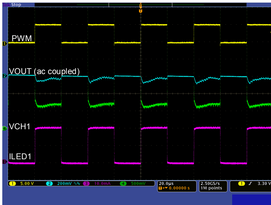
Figure 8. Typical operating waveforms (FPWM = 25 kHz, 50% duty)
