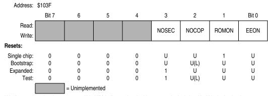
U indicates a previously programmed bit. U(L) indicates that the bit resets to the logic level held in the latch prior to reset, but the function of COP is controlled by the DISR bit in TEST1 register.
