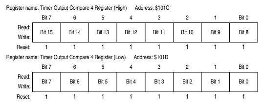
Figure 9-11. Timer Output Compare 4 Register Pair (TOC4)
