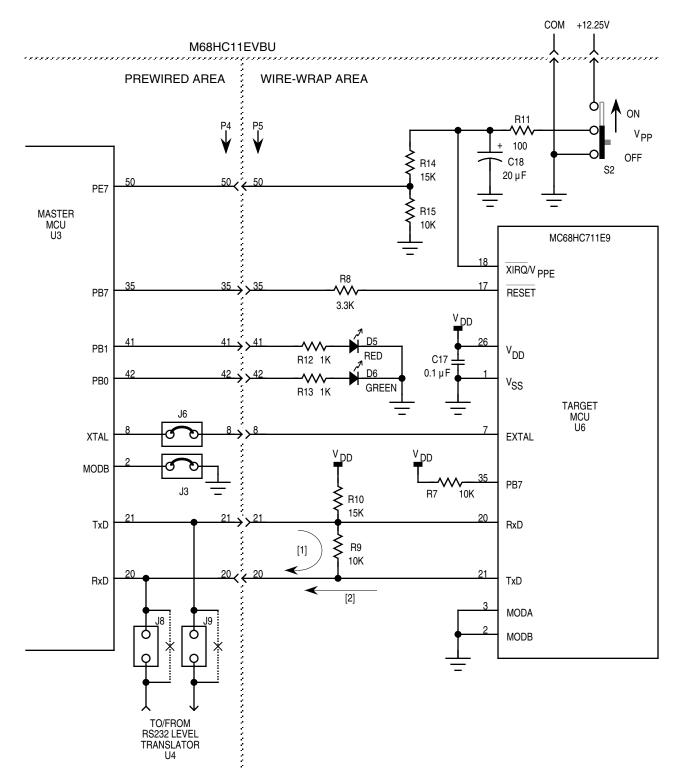
Figure 6. MCU-to-MCU EPROM Duplicator Schematic
