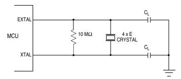
Figure 1-9. Common Parallel Resonant Crystal Connections
