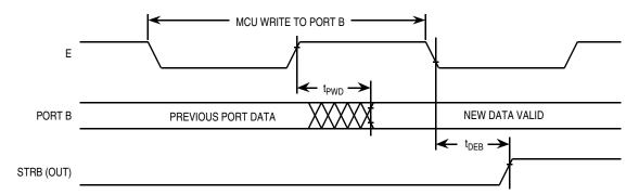
Figure 10-10. Simple Output Strobe Timing Diagram
