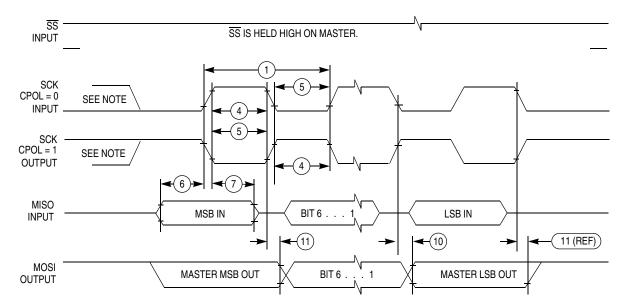
Note: This first clock edge is generated internally but is not seen at the SCK pin.
