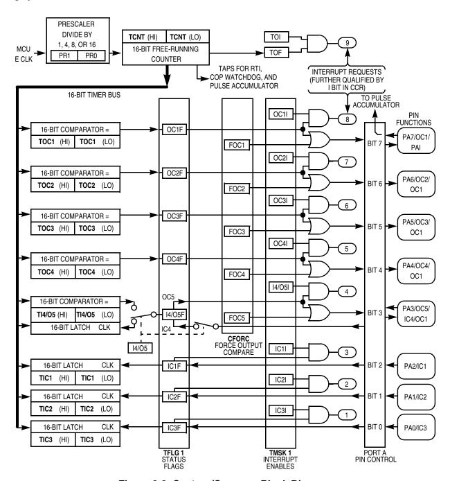
Figure 9-2. Capture/Compare Block Diagram
