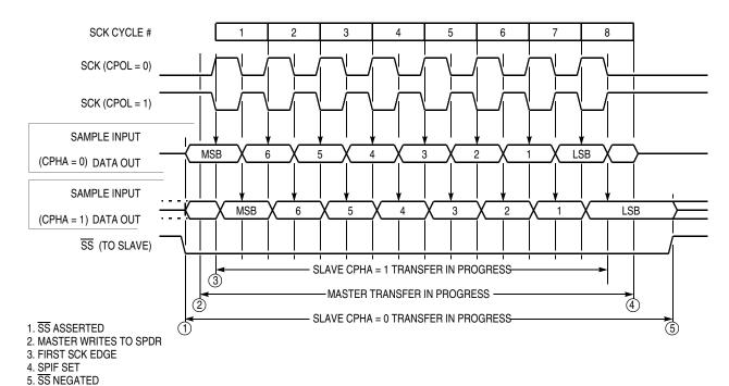
Figure 8-2. SPI Transfer Format
