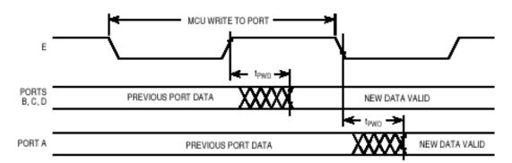
Figure 10-8. Port Write Timing Diagram
