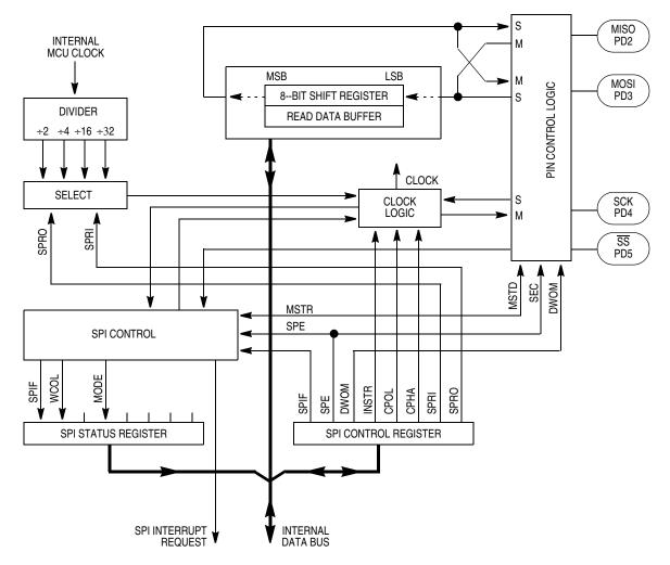
Figure 8-1. SPI Block Diagram
