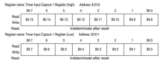
Figure 9-4. Timer Input Capture 1 Register Pair (TIC1)
