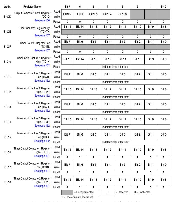
Figure 2-7. Register and Control Bit Assignments (Sheet 2 of 6)
