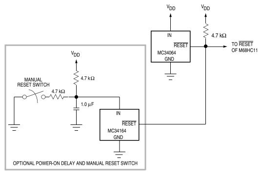
Figure 1-8. External Reset Circuit with Delay
