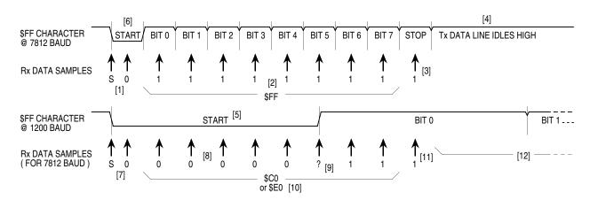
Figure 2. Automatic Detection of Baud Rate
