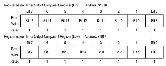
Figure 9-8. Timer Output Compare 1 Register Pair (TOC1)
