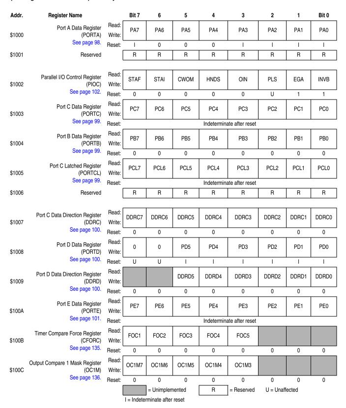
Figure 2-7. Register and Control Bit Assignments (Sheet 1 of 6)
