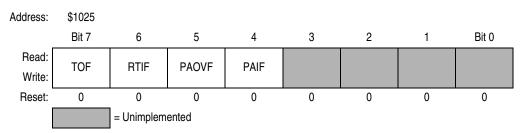
Figure 9-28. Timer Interrupt Flag 2 Register (TFLG2)
