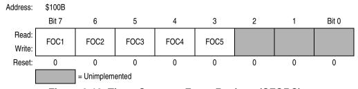
Figure 9-12. Timer Compare Force Register (CFORC)
