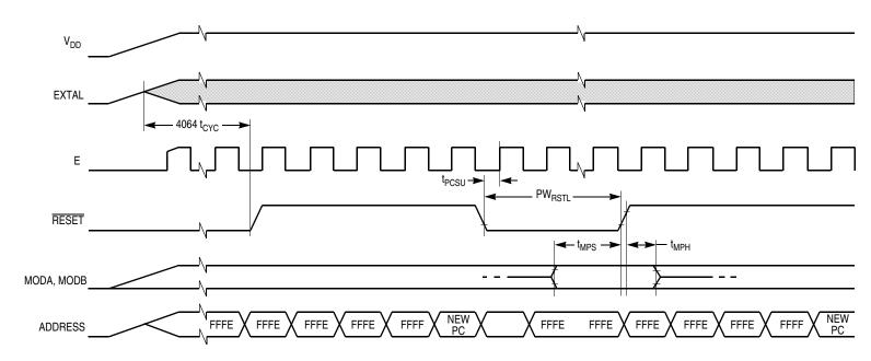
Figure 10-3. POR External Reset Timing Diagram
