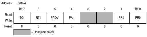
Figure 9-27. Timer Interrupt Mask 2 Register (TMSK2)
