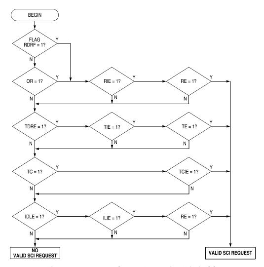
Figure 5-7. Interrupt Source Resolution Within SCI
