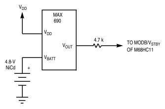
Figure 2-8. RAM Standby MODB/V<sub>STBY</sub> Connections
