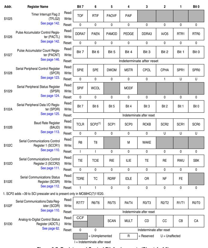
Figure 2-7. Register and Control Bit Assignments (Sheet 4 of 6)
