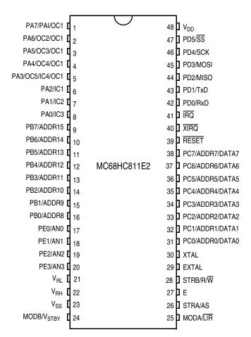
Figure 1-6. Pin Assignments for 48-Pin DIP (MC68HC811E2)
