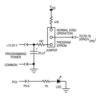
Figure 8. PC-to-MCU Programming Circuit
