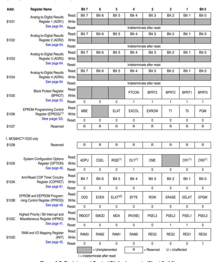
Figure 2-7. Register and Control Bit Assignments (Sheet 5 of 6)
