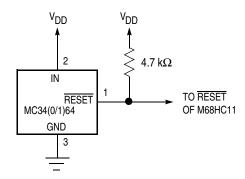
Figure 1-7. External Reset Circuit
