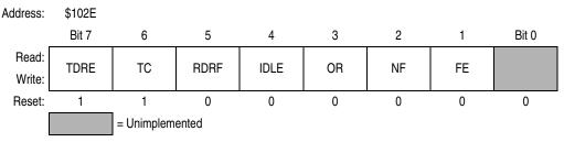
Figure 7-6. Serial Communications Status Register (SCSR)
