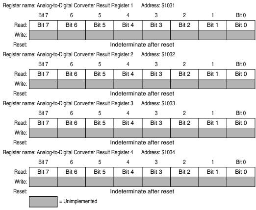
Figure 3-6. Analog-to-Digital Converter Result Registers (ADR1–ADR4)
