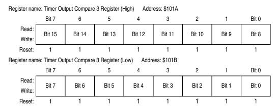
Figure 9-10. Timer Output Compare 3 Register Pair (TOC3)
