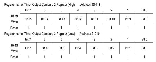
Figure 9-9. Timer Output Compare 2 Register Pair (TOC2)
