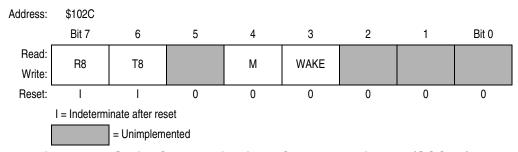
Figure 7-4. Serial Communications Control Register 1 (SCCR1)
