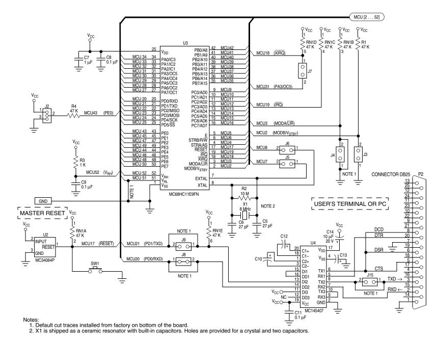
Figure B-1. EVBU Schematic Diagram
