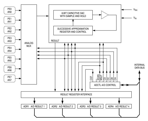
Figure 3-1. A/D Converter Block Diagram
