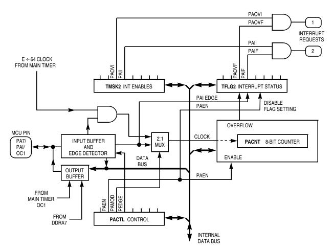
Figure 9-24. Pulse Accumulator
