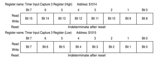
Figure 9-6. Timer Input Capture 3 Register Pair (TIC3)
