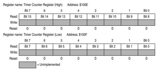
Figure 9-15. Timer Counter Register (TCNT)
