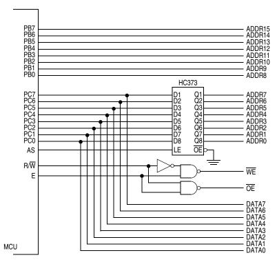
Figure 2-1. Address/Data Demultiplexing
