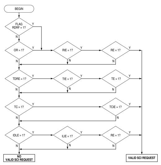
Figure 7-10. Interrupt Source Resolution Within SCI
