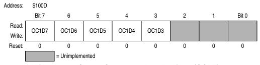
Figure 9-14. Output Compare 1 Data Register (OC1D)
