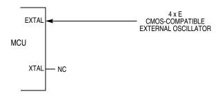
Figure 1-10. External Oscillator Connections
