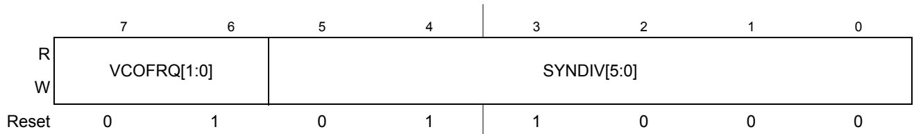
Figure 7-5. S12CPMU_UHV_V6 Synthesizer Register (CPMUSYNR)
