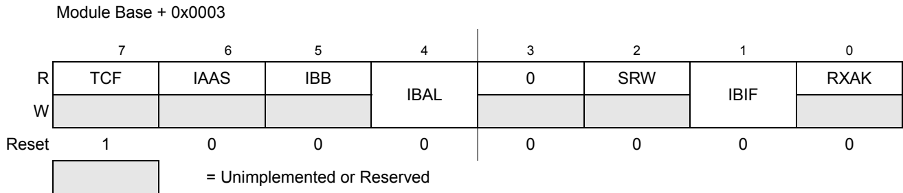
Figure 13-7. IIC Bus Status Register (IBSR)
