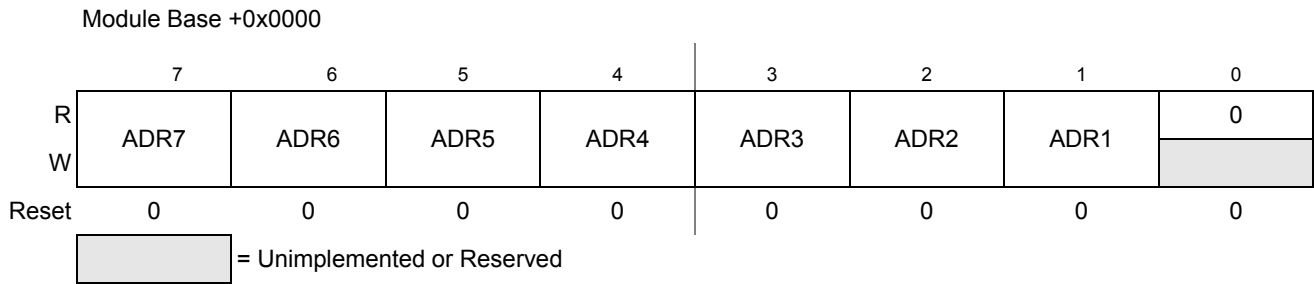
Figure 13-3. IIC Bus Address Register (IBAD)
