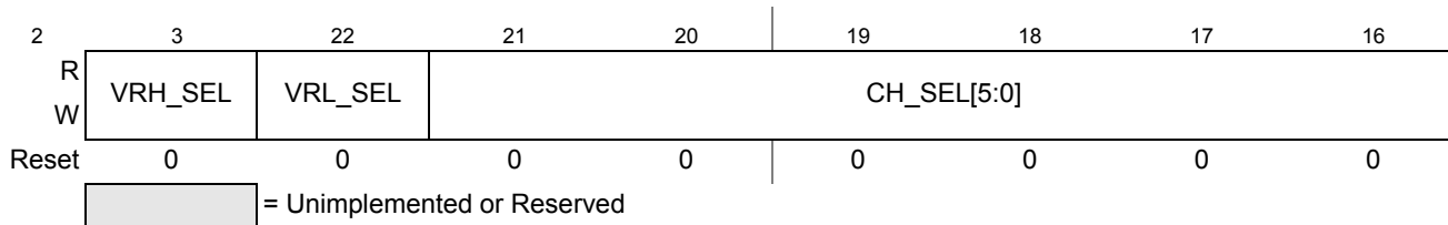
Figure 10-19. ADC Command Register 1 (ADCCMD_1)
