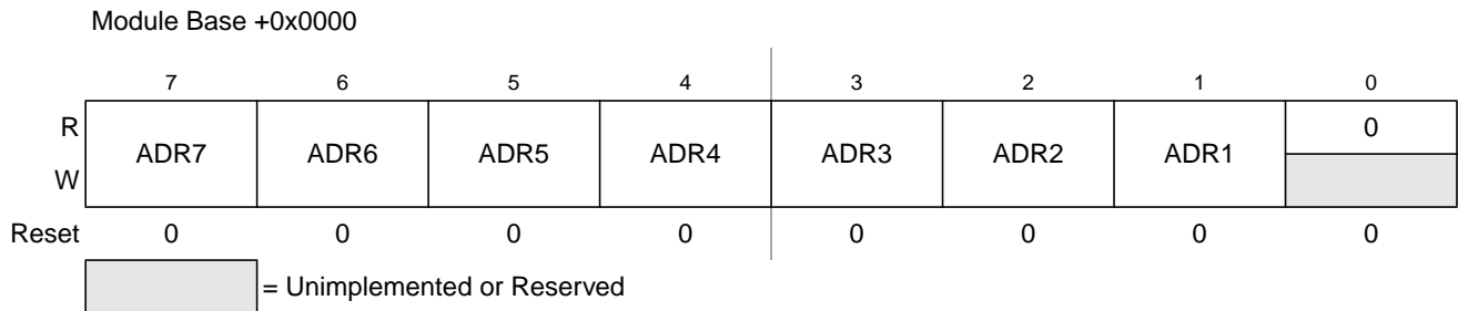
Figure 12-3. IIC Bus Address Register (IBAD)
