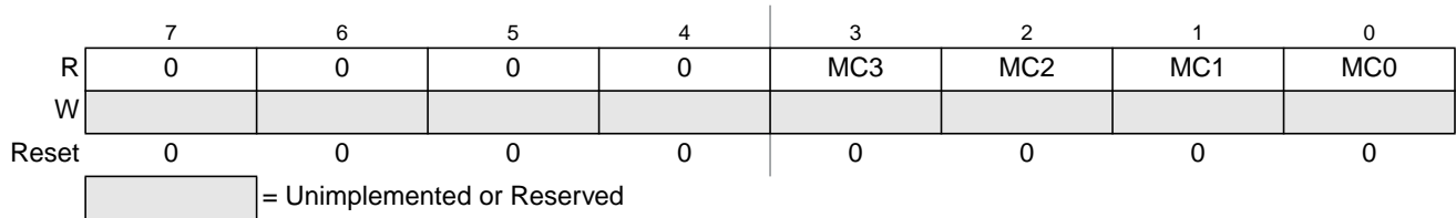
Figure 6-12. Debug Match Flag Register (DBGMFR)
