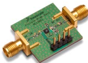
Figure 12. Typical Assembled Evaluation Board with SMA Connectors
