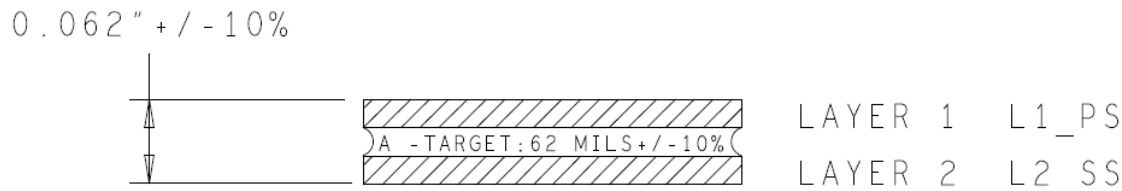
Figure 17. FRDM-CR20A PCB stackup cross-section (four layer)
