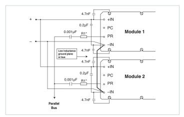
**Figure 9** — AC coupled single-wire interface
