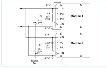
**Figure 10** — Transformer-coupled interface
