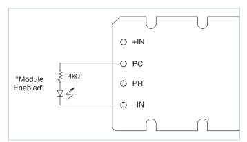
Figure 4 — LED on-state indicator
