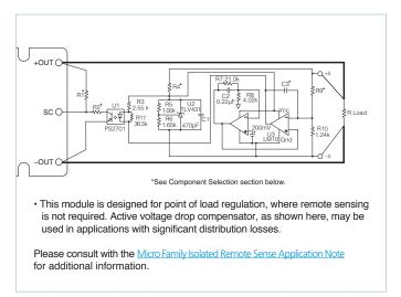
**Figure 12** — Voltage drop compensation
