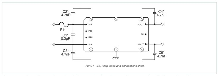
Figure 1 — Basic module operation requires fusing, grounding, bypassing capacitors.\* See Maxi, Mini, Micro Design Guide.
