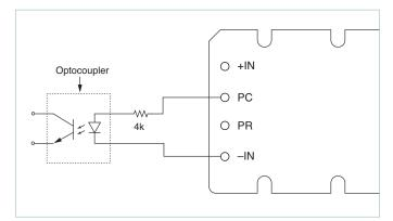
Figure 6 — Isolated on-state indicator
