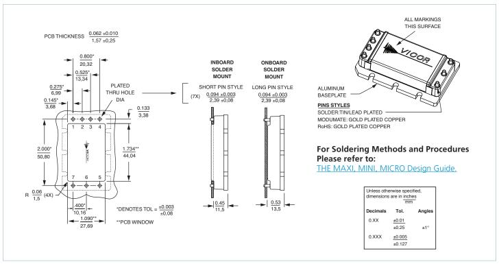
Figure 14 — PCB mounting specifications
