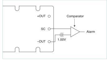
Figure 7 — Secondary side on-state indicator
