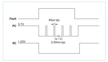
Figure 5 — PC/SC module alarm timing
