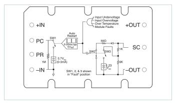
Figure 3 — PC/SC module alarm logic
