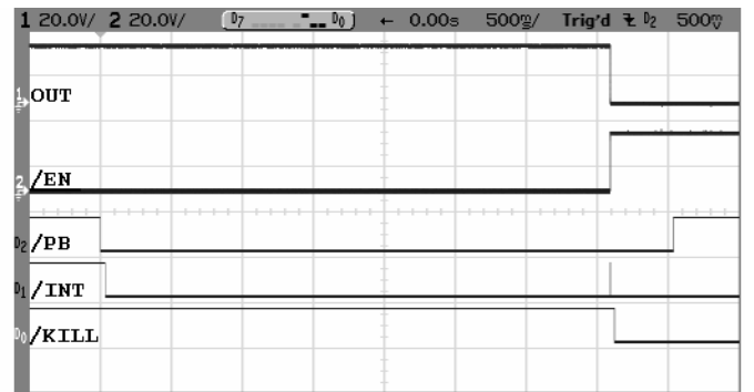
(b) Push Button Turn Off (PDT = 0.47µF, 500ms/div)
