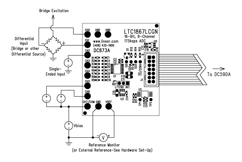
Figure 1. Connection Diagram
