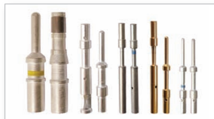
The CA Bayonet contacts incorporate copper alloy plated with a hard silver finish (optional gold) and guarantee at least 500 mating cycles. All solder contacts feature a special passivation to comply with RoHS requirements.
