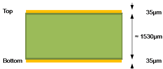
Figure 4-6. PCB layer stack.
