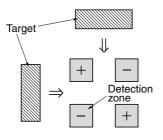
2) Direction As detailed on the diagram, please install the sensor so that the expected trespassing direction corresponds to the axis X or axis Y.
