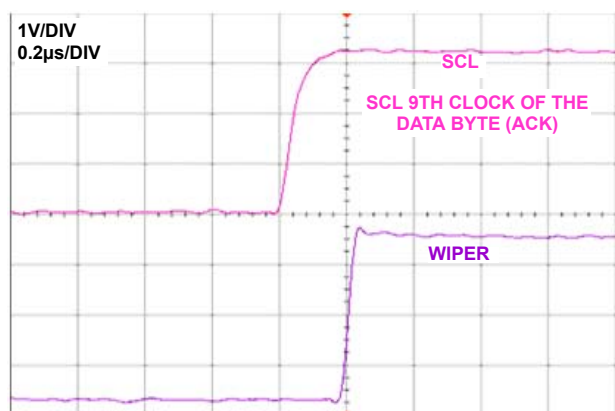
FIGURE 21. WIPER LARGE SIGNAL SETTLING TIME
