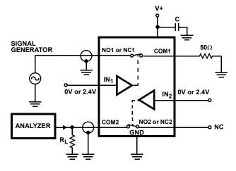
FIGURE 6. CROSSTALK TEST CIRCUIT
