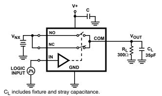
FIGURE 3C. MEASUREMENT POINTS (ISL84544 ONLY)
