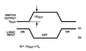
FIGURE 2A. MEASUREMENT POINTS
