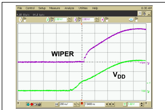
FIGURE 2-14: 2.1 kΩ – Power-Up Wiper Response Time.
