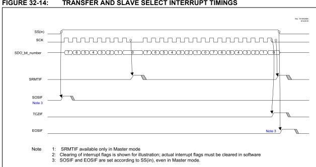
FIGURE 32-14: TRANSFER AND SLAVE SELECT INTERRUPT TIMINGS
