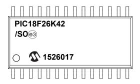
28-Lead SSOP (5.30 mm)
