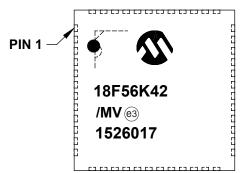
48-Lead TQFP (7x7x1 mm)
