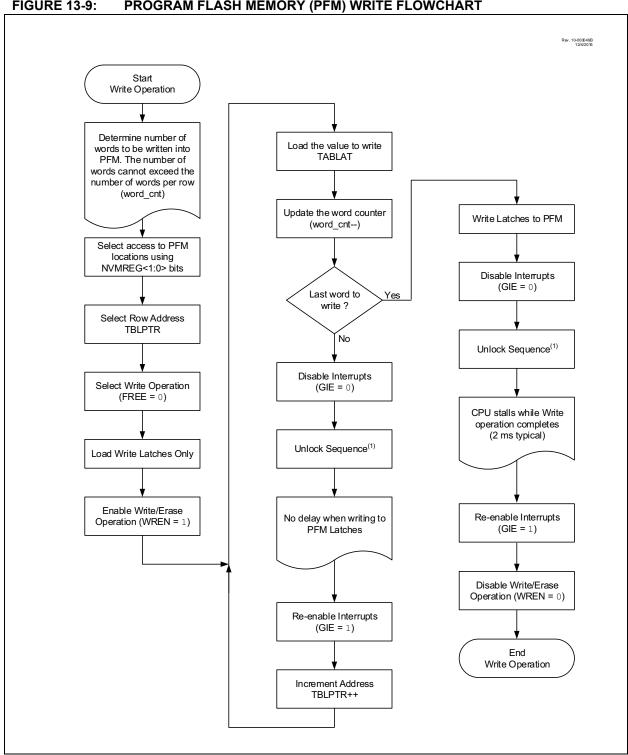
**FIGURE 13-9:** PROGRAM FLASH MEMORY (PFM) WRITE FLOWCHART
