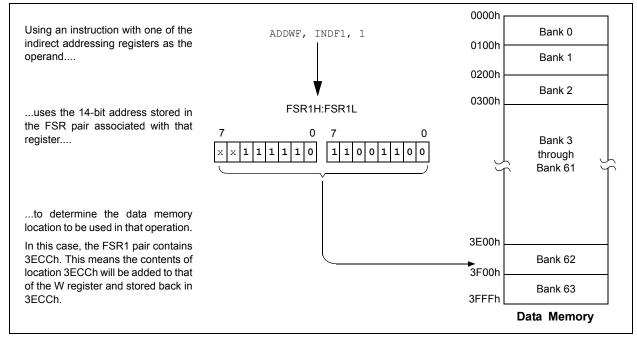
Operations on the FSRs with POSTDEC, POSTINC and PREINC affect the entire register pair; that is, rollovers of the FSRnL register from FFh to 00h carry over to the FSRnH register. On the other hand, results of these operations do not change the value of any flags in the STATUS register (e.g., Z, N, OV, etc.).
