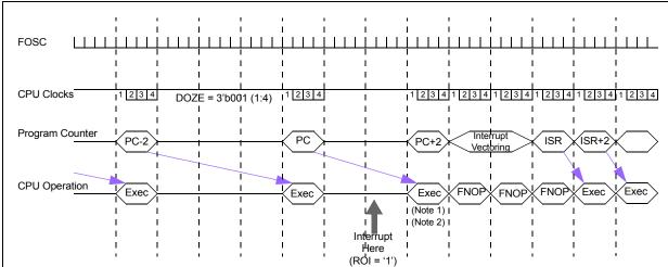
Note 1: Multicycle instructions are executed to completion before fetching the interrupt vector.
