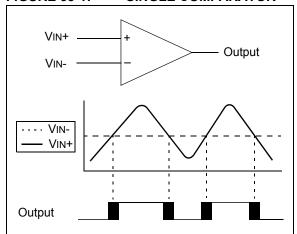
**Note:** The black areas of the output of the comparator represents the uncertainty due to input offsets and response time.
