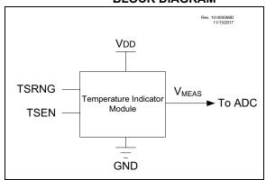
The output of the circuit is measured using the internal Analog-to-Digital Converter. A channel is reserved for the temperature circuit output. Refer to Section 36.0 "Analog-to-Digital Converter with Computation (ADC2) Module" for detailed information.
