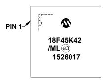
44-Lead TQFP (10x10x1 mm)
