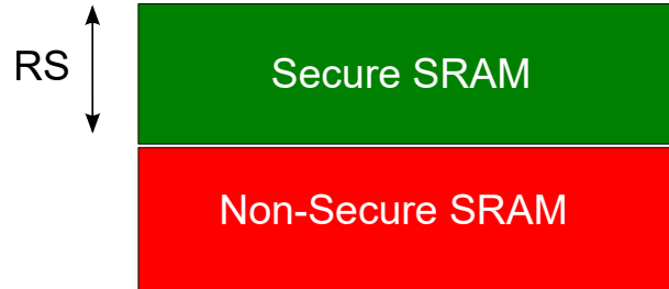
Figure 13-4. SAM L11 SRAM Memory Mapping
