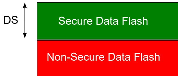
Figure 13-3. SAM L11 Data Flash Memory Mapping
